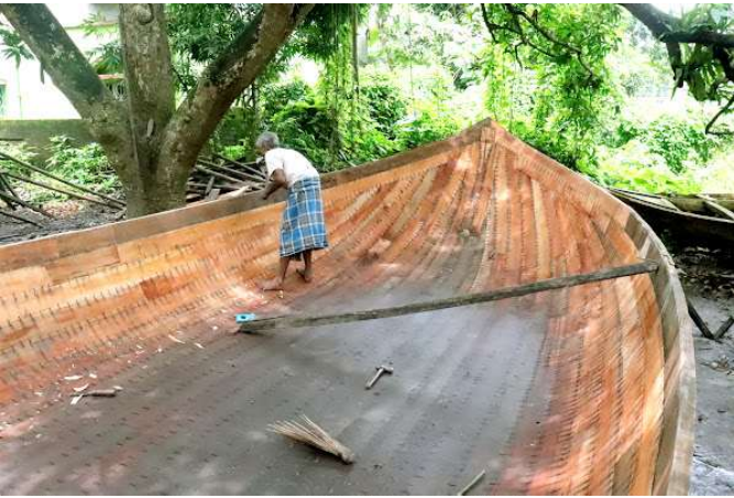
Figure 9 : Sambhu Barik, 72, a traditional boat maker of Balagarh, Hugli district, West Bengal. Balir Nouko (specifically made to carry sand from river bed) is one of the popular boat of Balagarh. Length varies from 30 to 50 feet.
