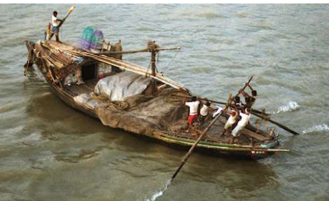
Figure 5 : Mahajoni Nouka, supplier of goods through waterways. Carrying capacity ranges from 1000 to 2000 mounds. Shell built, stapled and rivetted boat propelled by oar and square sail.
