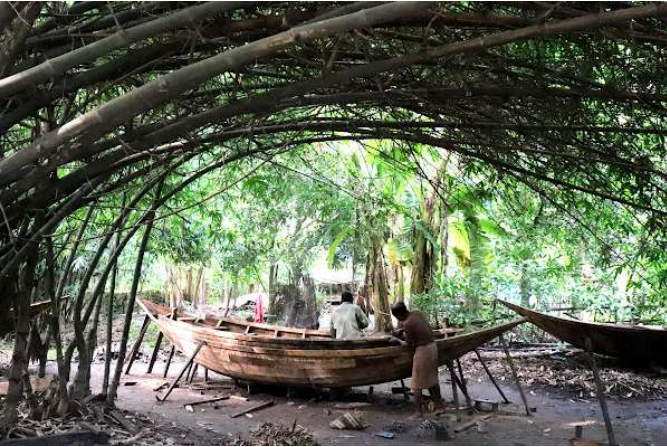
Figure 1: Living Tradition. Traditional boat makers use bamboo grove as the ideal place for boat making. Shed of the bamboo grove is preferred as the climate in this part of the world is hot and humid. Not only that, bamboo is also an important tool of boat making. Balagarh in Hugli district is a commercial boat building centre of Bengal where Rajbansi boat makers (a fishing caste of Bengal) are the boat makers who build boats throughout the year and keep it in their boat building shed for sale.
