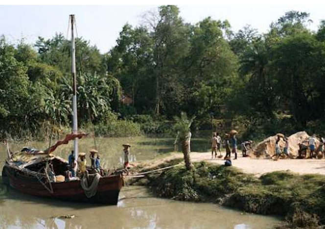
Figure 6 : Sultani, a skeleton build boat of Medinipur district propelled by lug sail. Due to incorporation of engine, sailing boats are now without any mast. A boat popularly known as medinipuri boat.
