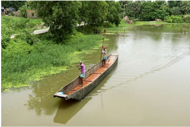
Figure 4 : Shalti, a traditional wooden boat of Lower Gangetic Plain. Long and narrow boats are used to carry all kinds of goods through narrow channels of the Sundarbans. Method of propulsion is punting.
