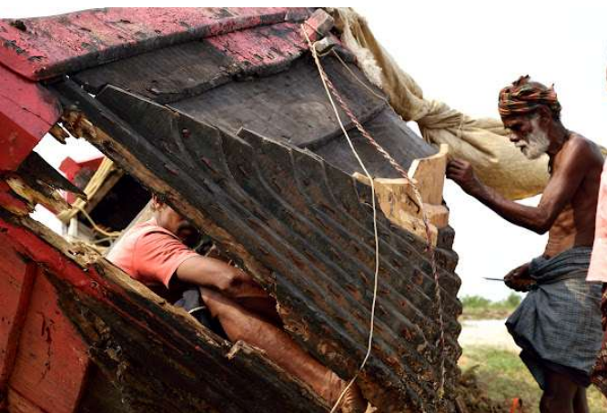
Figure 8 : Gangadhar Pattayit, 69 (Head Mistiri) chief boat maker of Kasafal region, Odisha. He acquired craftsmanship from his guru (teacher) and has taught the skill to 20 disciple (sishyo). The boat he is repairing was made by his guru 30 years ago. Quality of wood, craftsmanship and maintenance are the key factors for the life of a boat.
